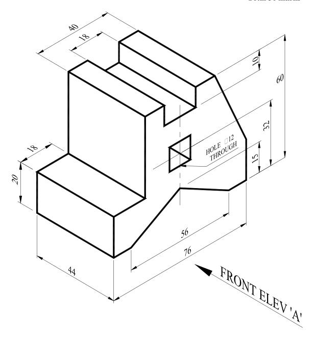
2. The figure below shows three views in first angle orthographic projection and an oblique view of a shaped block.
